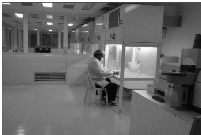
Figure 1. Class 100 clean room with class 10 laminar flow work benches of Ultra Trace Analytical Laboratory at NCCCM
